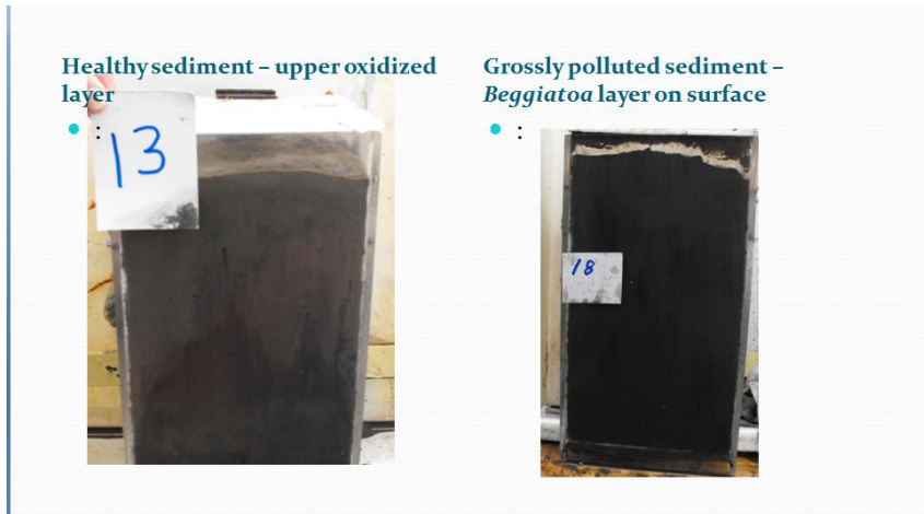
Figure 12. Sediment profile images with oxidized surface sediment (left) and no oxic layer (right).
